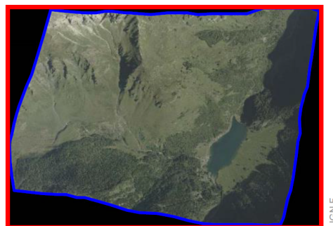
Figure 9 – footprint and bounding box of an orthoimage (respectively in blue and red)
