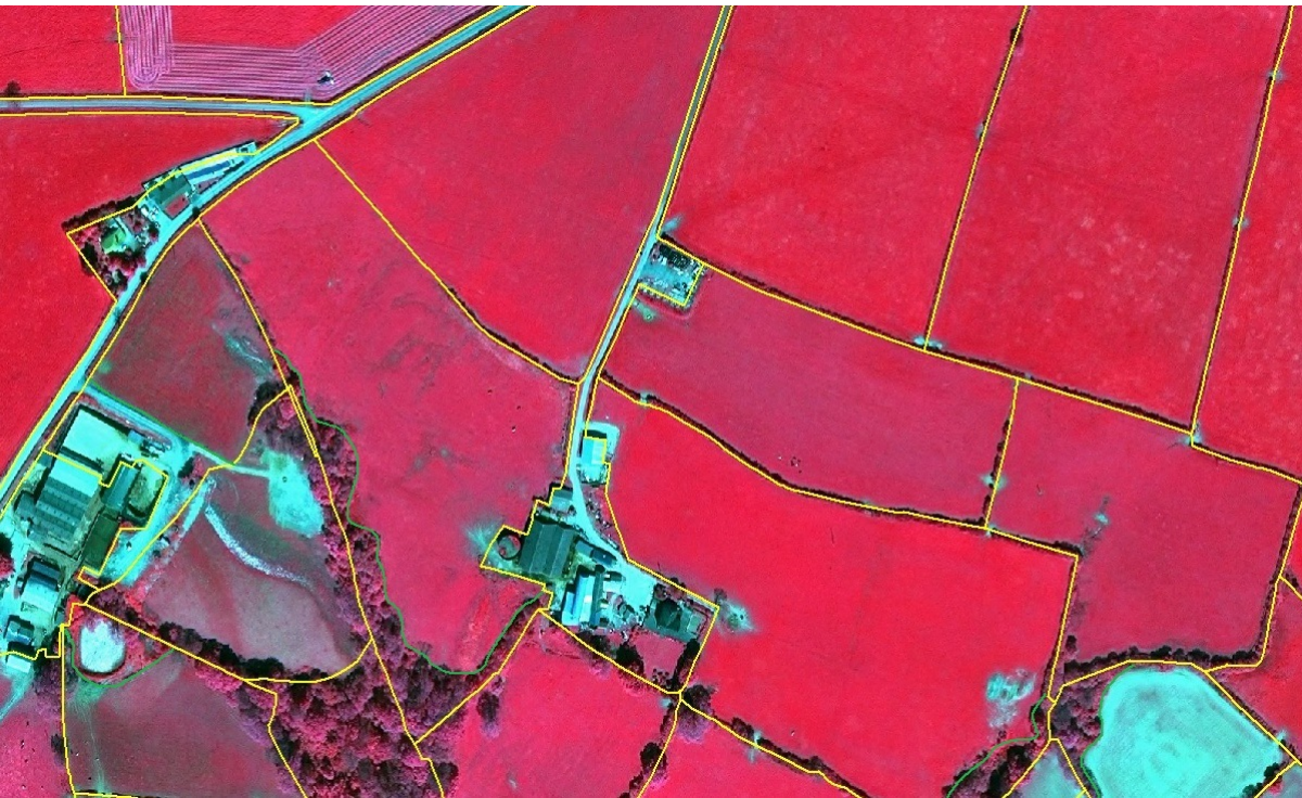
Figure 30: "topographical" reference parcels; units of land derived from selected topographical map features (yellow line) with delineation of agricultural land (green line) therein.
