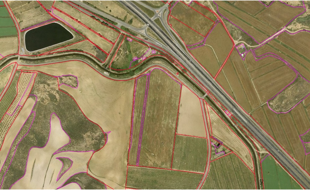
Figure 29: "cadastral" reference parcels; cadastral parcels (red lines) with delineation of agricultural land therein (magenta lines).
