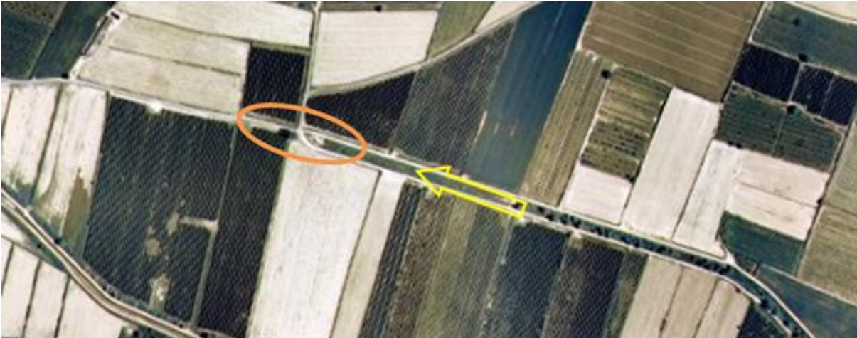
Figure 21 - The watercourse vanishes meaning it is impossible to position it. (Arrow indicates water flow direction)
