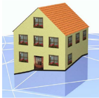
Figure 34: The terrain intersection is shown in black
