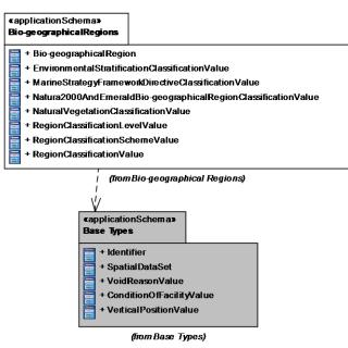
Figure 4 – UML class diagram: Overview of the Bio-geographicalRegions application schema
