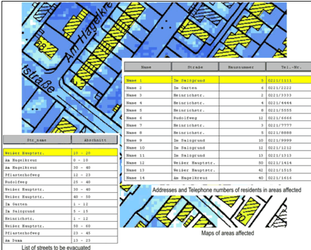
Figure 3.2-10: Calculated flooded areas and table of street segments (aggregation of addresses) and citizens are affected (IVU) 4
